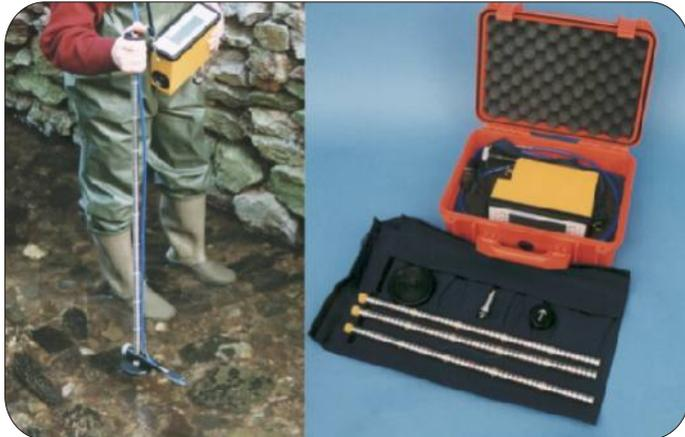
The Model 801 Electromagnetic Flow Meters measure the speed of water in Open Channel environments with exceptional accuracy. Two sensor types are available, to suit different application requirements, but both offer excellent durability, reliable accurate data, and are suitable for use in clean water and dirty or difficult environments.
